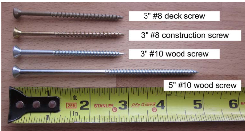
Figure 3 : Strapping attachment screws
