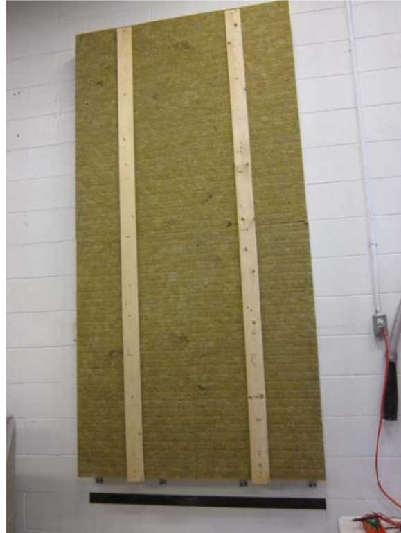
Figure 2 : Roxul insulation attached to wall frame ready for test
